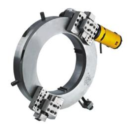
ISD Models high-performance carbon brush electric drive which is powerful and steady, Metabo motor drive; Split framerate-rust steel body, optional aluminum alloy made; Install on the outside of pipe fast and steady; Automatic feed mode; Cutting and beveling at the same time; High precision, operate simple and secure.
