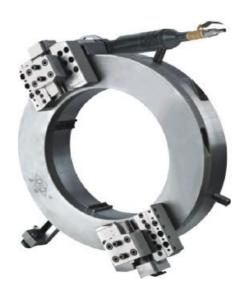
GPD Models pneumatic motor are drive with strong force and low noise; Split frame, Can be quickly installed on the outside of pipe and rigidly; Automatic tool feeding; Cutting and beveling at the same time; Steel main body, or aluminum alloy body; High precision machining, easy operation. Suitable for explosion-proof environment.
