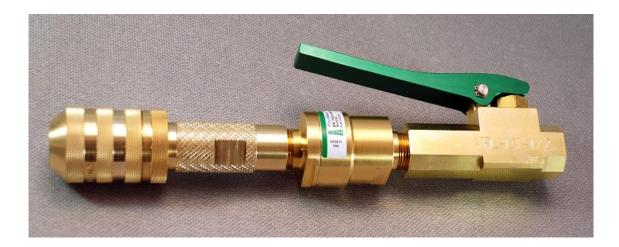
The PL Holder is an all brass holder that incorporates a hardened steel lock ring to hold the Lance Pipe with a Viton rubber Grommet to provide a positive seal for the oxygen supply.
